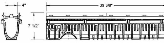
100C HD Presloped Channel with DI Frame (Preslope Upgrade)
